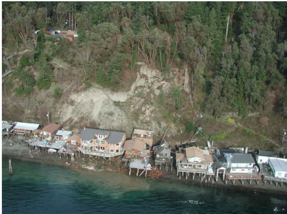
Figure 3—Salmon Beach landslide area, near Tacoma, after the 2001 Nisqually earthquake. Puget Sound is in the foreground (Photo from Bray and others, 2001)
